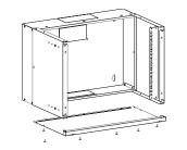
Assemble bottom sheet with special plastic rivets Note: the bottom sheet has no fan cutouts
