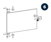
Hinges and lock parts are pre-assembled on the glass door Note: take care not to damage the glass
