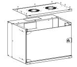
Assemble roof sheet with special plastic rivets Note: the roof sheet has fan cutouts
